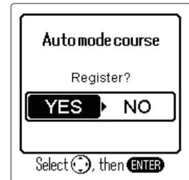
**5** Select "YES". Registration starts. With the message "Finished" on the LCD, the process of registration is completed.
